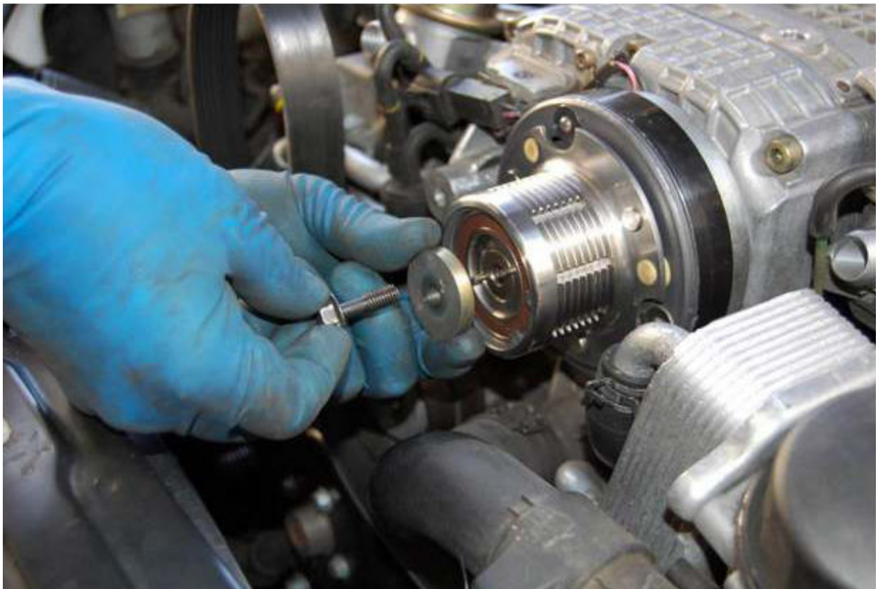
Step 5- Remove the bolt and washer from the front of the pulley
